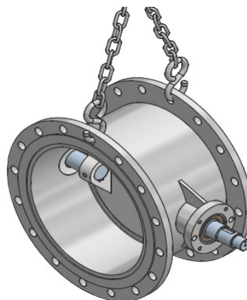
Figure 4-2: Attachment to the flange holes
